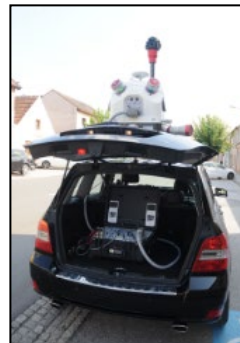
RIEGL VMX-2HA equipped with FLIR Ladybug® 5+ camera
