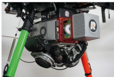
RIEGL miniVUX-SYS with APX-20 UAV RIEGL miniVUX-1UAV LiDAR sensor equipped with APX-20 UAV
