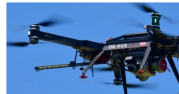
RiCOPTER-M equipped with ADS-B/Mode-S transponder
