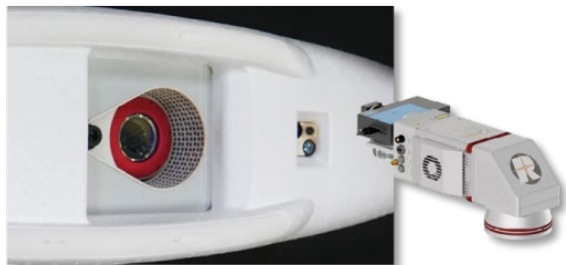
RIEGL miniVUX-SYS with APX-15 UAV Delair DT26X fixed-wing integration example with RIEGL miniVUX-1DL LiDAR sensor equipped with APX-15 UAV
