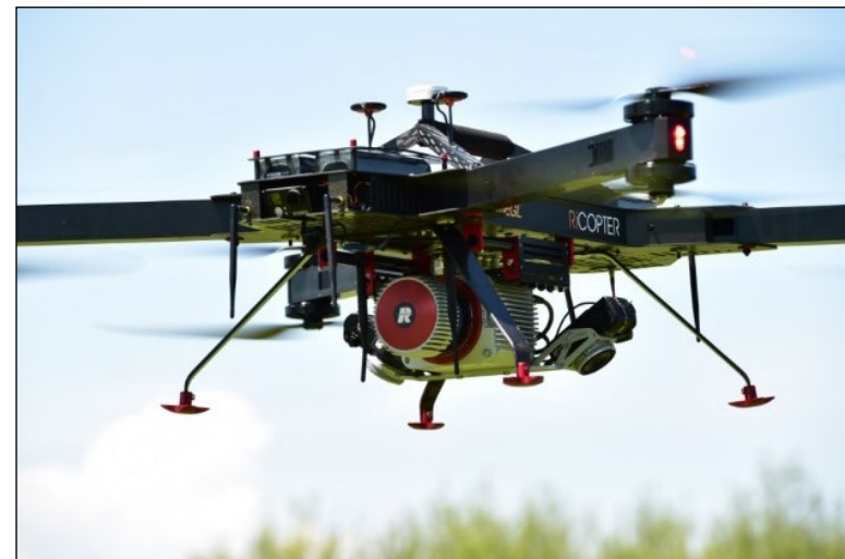
RiCOPTER-M equipped with ADS-B/Mode-S transponder
