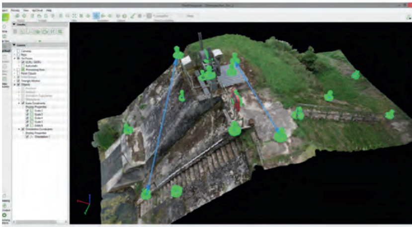
▲ Figure 3: Dam monitoring and inspection – photogrammetry model of a dam within Pix4D.
