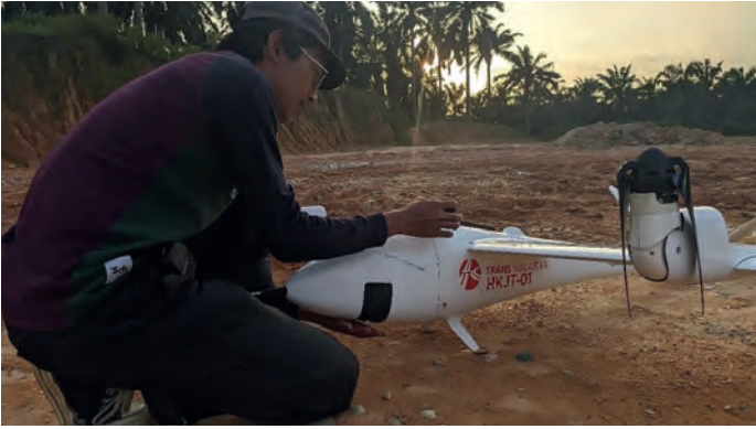
▲ Preparing for the UAV-Lidar survey of the Betung to Jambi section. (Image courtesy: Hutama Karya)
