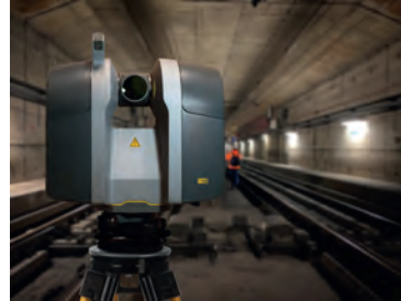
▲ The Trimble TX8 enables more than one track to be scanned at the same time.
