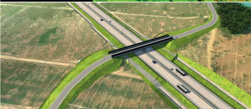
▲ DTM of the Betung to Jambi section (top) and BIM in InfraWorks software using the Lidar DTM of the Betung to Jambi section (bottom). (Image courtesy: Hutama Karya)
