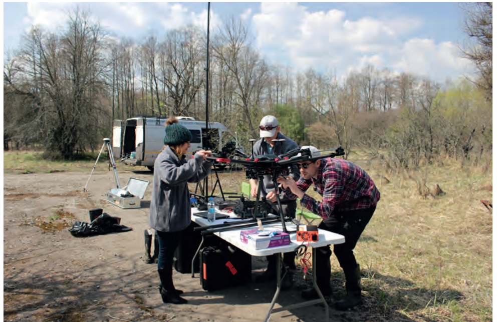
▲ M600 with LidarPod being set up for flight. (Image courtesy: Yannick Verbelen, Bristol robotics team)
