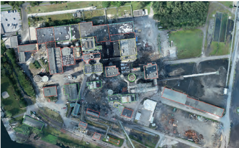
▲ Figure 3: Orthophotograph with CAD drawing overlaid.
