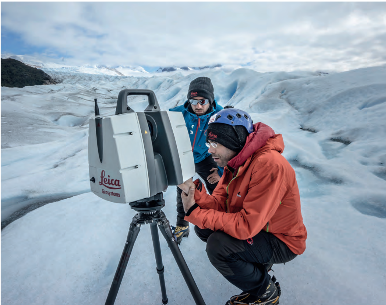
▲ The Leica ScanStation P40 was used to capture 3D data within and near the entrance of a cave at the base of the Perito Moreno glacier, Argentina. (Image courtesy: Alessio Romeo)
