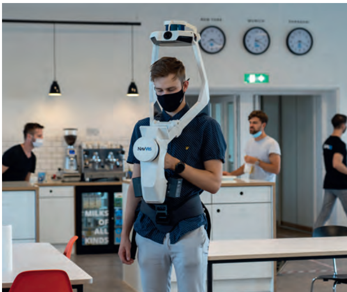
▲ NavVis VLX has SLAM capabilities and can also tie into measurement points in GNSS-denied environments.
