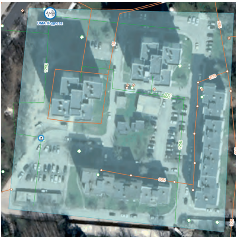
▲ A DMA zone coloured blue indicates that the collected data is within the pre-defined norms.
