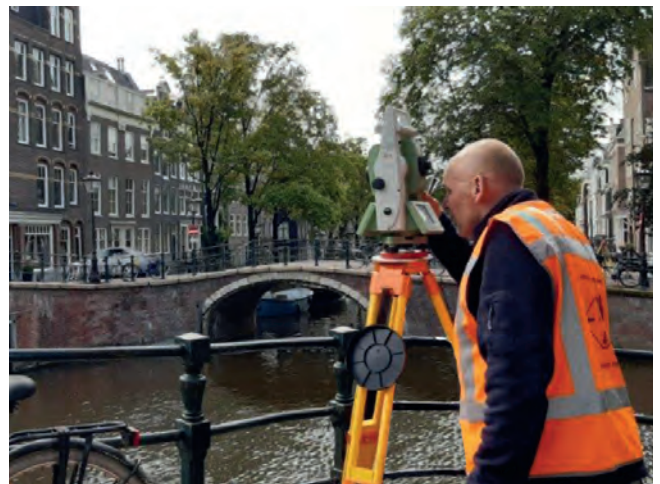
▲ Fugro is monitoring hundreds of bridges and kilometres of quay walls in Amsterdam, some of which have reached the end of their structural lifespan.
